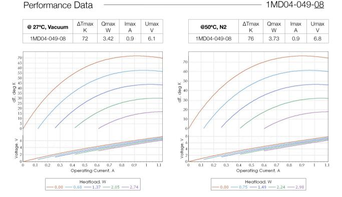
**Note**: Performance data is specified at optimal optimal conditions (TEC hot side is stabilized at ambient temperature). Any heatsink thermal resistance is not included into estimations. Use TECCad Software for estimations under different conditions.
